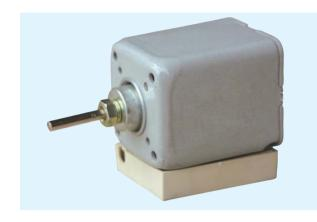
**Undervoltage Release**: Undervoltage release is used in opening air type circuit breaker due to low voltage or phase disconnection. There are two types of low voltage releasers as instant opening and delayed opening types. Delayed type undervoltage release has 1 sec., 2 sec. and 5 sec. delayed models and accuracy class is 15%.
